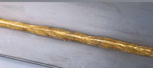
MIG pulsed brazing of thin sheets
